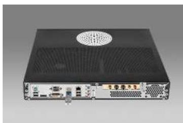
on the left and analogue connections on the right. The unit comes standard with a Xonar Essence board by ASUS although my unit had the optional DMA-03 analogue preamp board (\$1,895 additional cost). Mayerthaler told me the DMA-03 is vastly superior than the Xonar. The unit is powered by an external supply.
