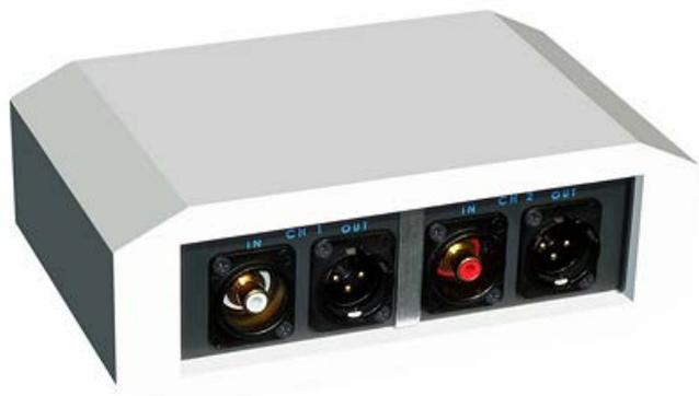
The special external and passive transformer DMA 04 is available as an optional accessory. The DMA 04 transformer allows the conversion of the unbalanced RCA output from the DMA 03 High-End Sound Module to a high-quality balanced XLR output with galvanic isolation.
